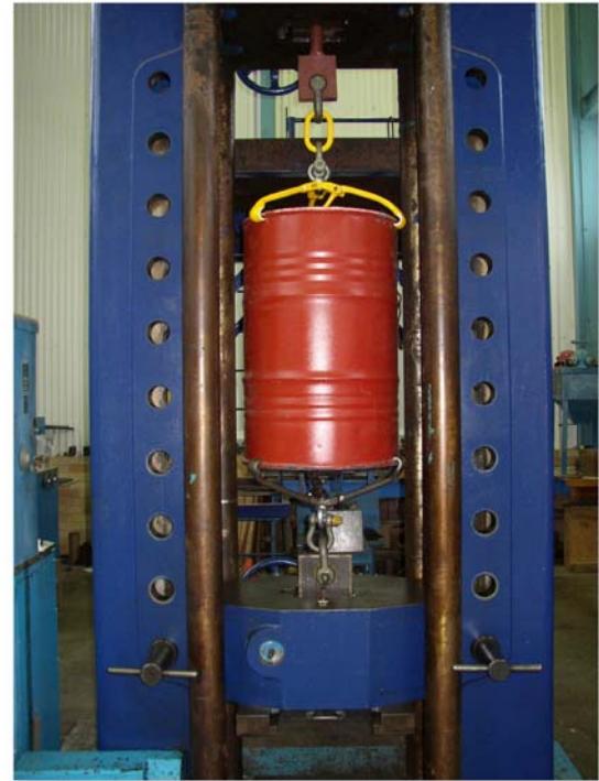
Drum-lifting device being tested at TestSafe
