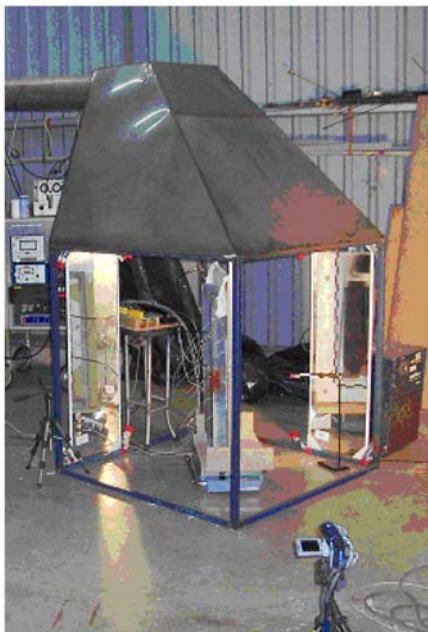
Furniture Calorimeter Hood (1.2 x 1.2m) commissioned at TestSafe for Masters Project
