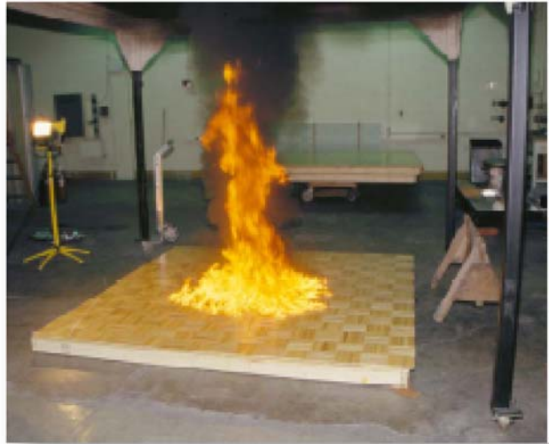
Full scale (2.4 x 2.4m) Furniture Calorimeter testing of burn patterns on parquetry floor by US National Institute of Justice
