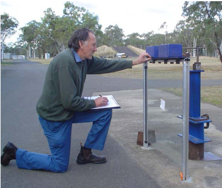
Laurie Gerisch testing glass railing at TestSafe.
