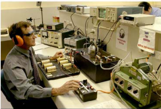
Garry Jeffery, Electrical Engineer, TestSafe Australia performing a spark test.
