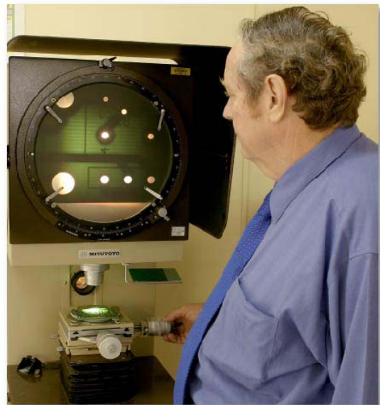
David Fraser, Electrical Engineer, TestSafe Australia performing a segregation distance measurement
