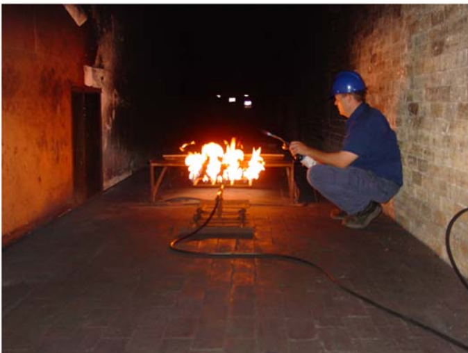
Michael Kovacs igniting the gas flame prior to testing the conveyor belt
