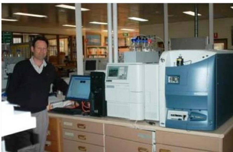
Robbie Geyer, Manager Thornleigh Laboratory standing next to the Triple Quadrupole Liquid Chromatograph Mass Spectrometer instrument
