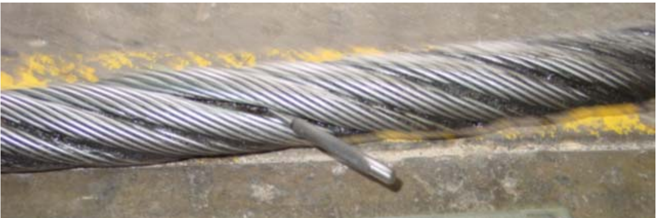
Typical Mine Drift Rope during examination.
