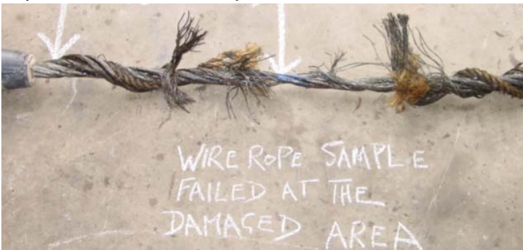
Mine Winder Rope following destructive rope testing
