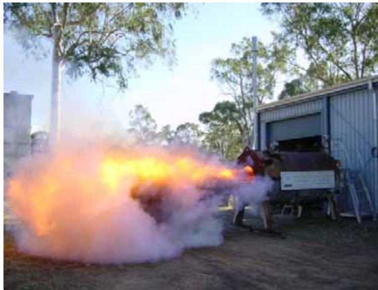
Partly confined dust/air explosion demonstration at TestSafe Australia Londonderry.
