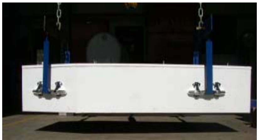
A cardboard coffin undergoing a lift test whilst filled with sandbags
