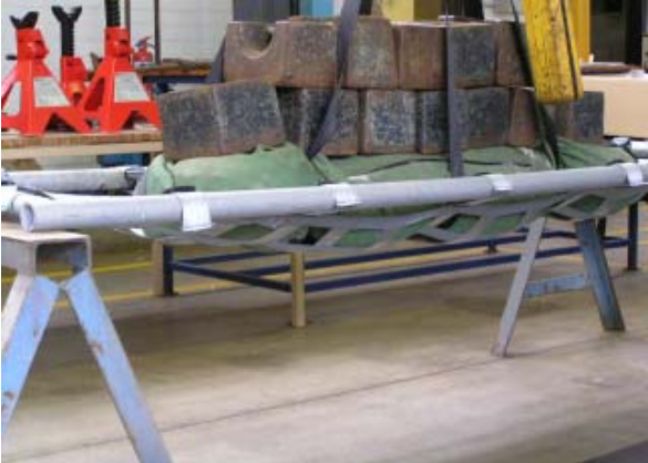
790 Kg Load Test on Grave Cover
