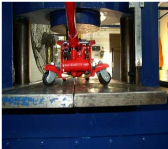
A trolley jack undergoing a load test in accordance with the Australian Standard
