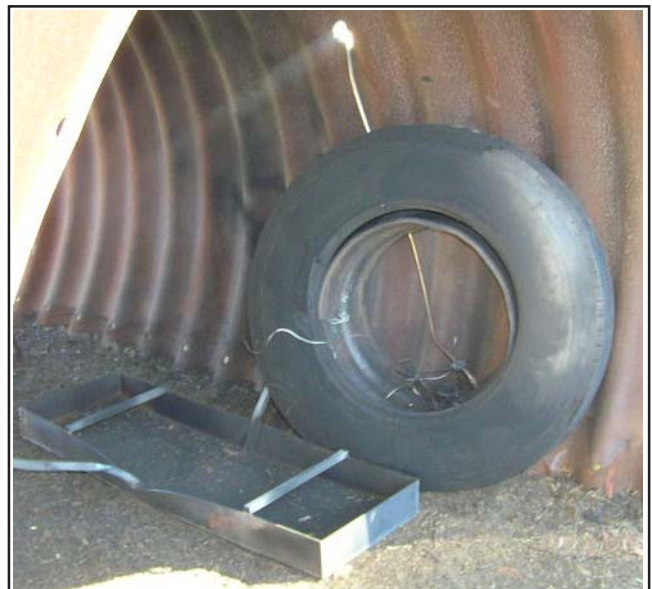
Tyre No 2 test - After Explosion
