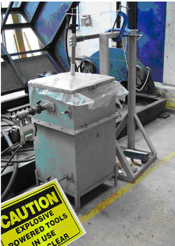
Power Tool being tested in Flameproof Testing Chamber
